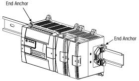
Note: For environments with greater vibration and shock concerns, use the panel mounting method described below, instead of DIN rail mounting.
